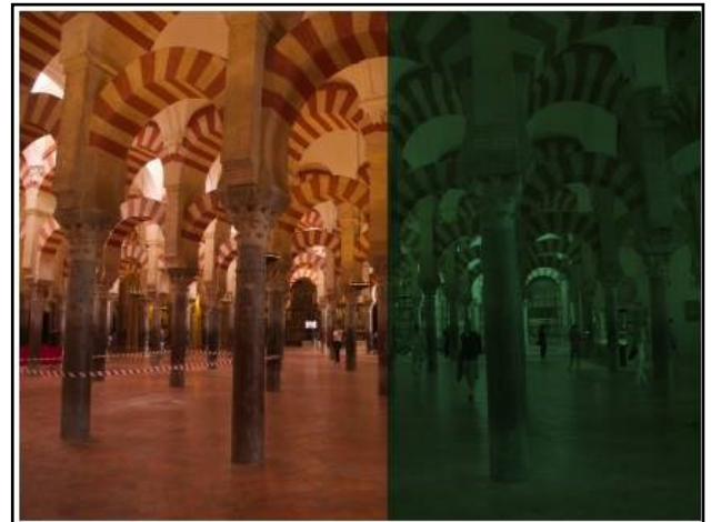
Figure 10. Image Before (Right) and After (Left) Demosaicing
