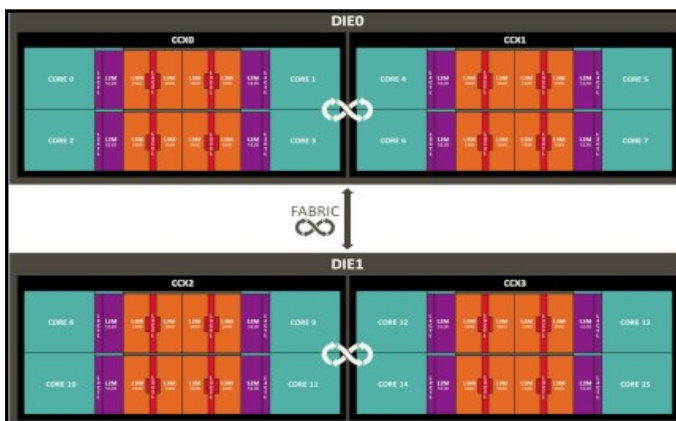
The layout for an AMD Threadripper processor using multiple CCXs. AMD
